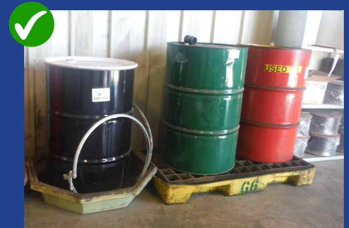
Keep oil and other fluids in containers with leak proof lids. Use secondary containment devices and store in a covered area.
