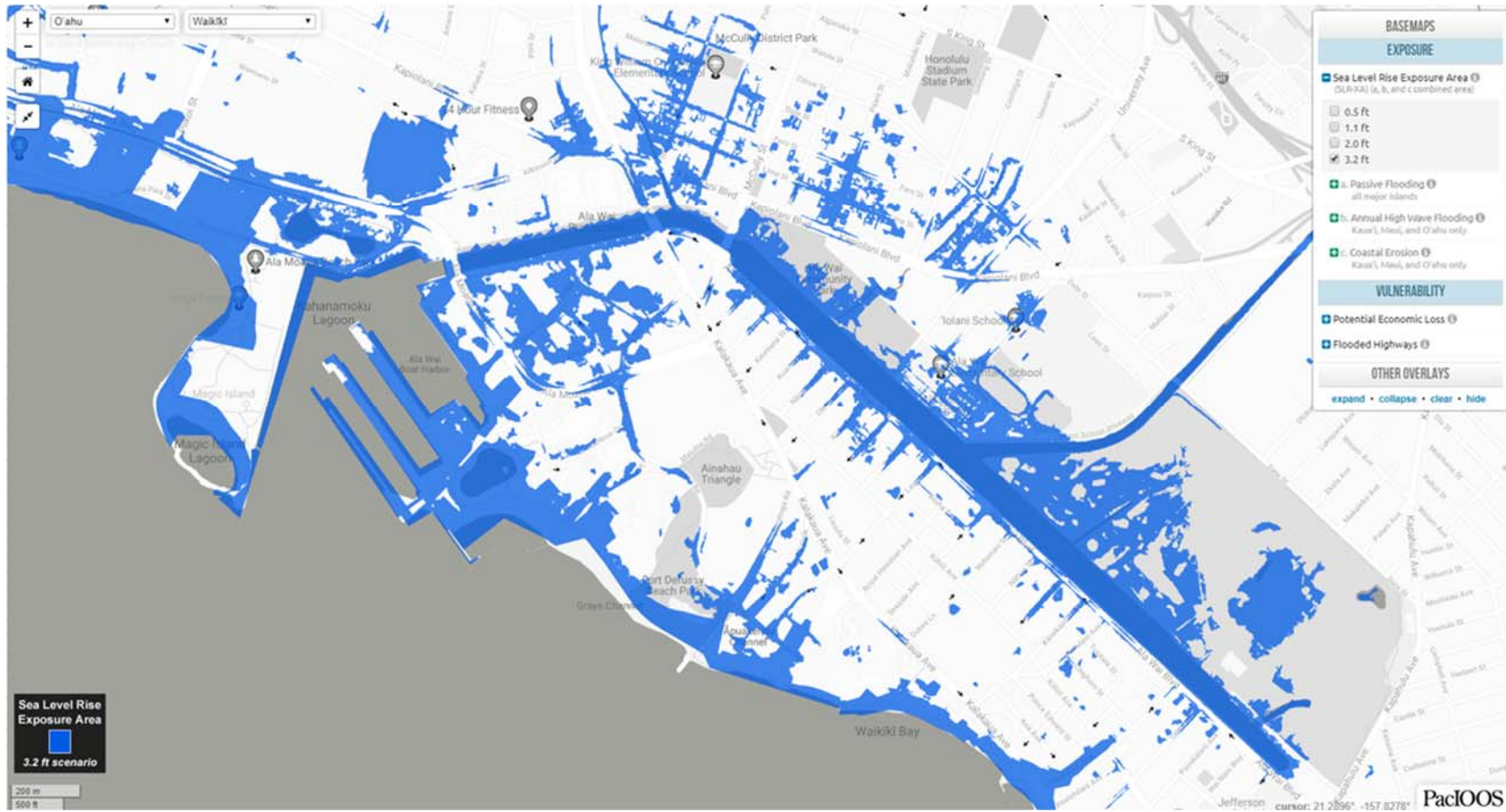
Figure 13 Land Area Change Under 3.2 Feet of Sea Level Rise Conditions
