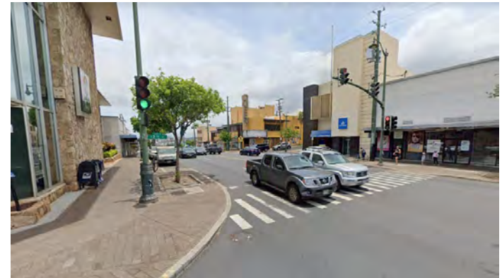
Curb extensions, Wai'alaie Ave.
